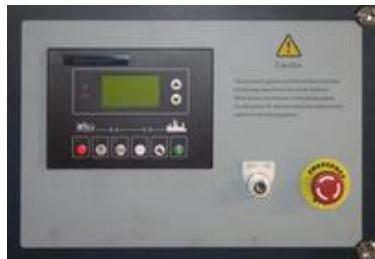
HKY-6110 control panel is fit for backpack structure and standing structure. This control panel is a panel which holds a HGM6110 made by Smartgen the professional module maker in China as its core intelligent control module. It has plenty friendly operation interface with many functions such as running parameter detecting, static, record, pre-alarm, Remote control, monitor & protection.
